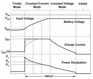
Figure 19. Typical Charge Curves Using a Constant-Voltage Adapter
